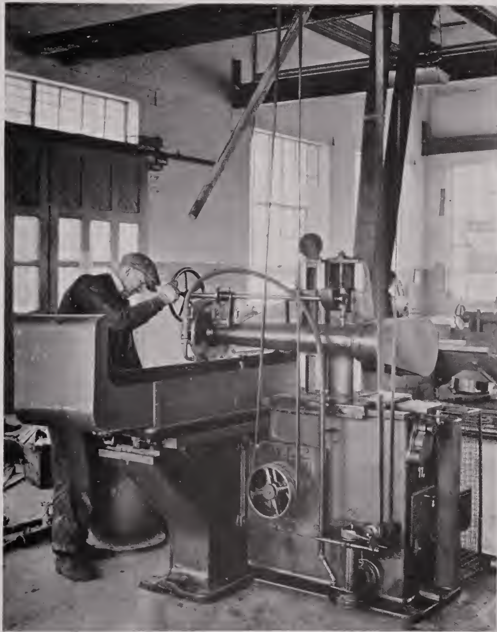
DIAMOND AUTOMATIC SURFACE GRINDER For smoothing die block surfaces.
